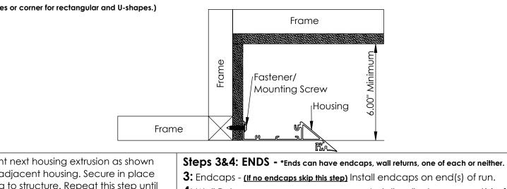
Step 2: (If single housing skp this step) Mount next housing extrusion as shown by sliding the provided joiners into the adjacent housing. Secure in place by tightening set screws. Mount housing to structure. Repeat this step until all housings are installed and mounted.
