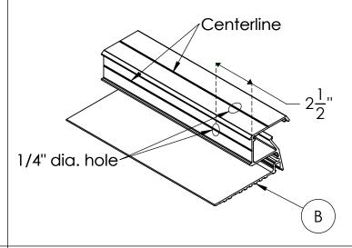
Step 3; Prepare the Ceiling: Construct false ceiling as shown below. Drill a 1/4" hole in the drywall to feed low voltage to the Luminaire (C). Ensure hole on drywall align with hole on housing. This hole can be either behind or above the intended position of luminaire depending on the path of low voltage wires.
