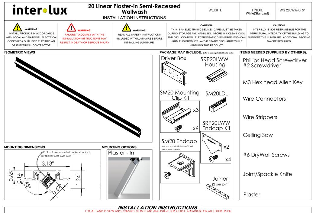
It is recommended to locate and lay out all components for each fixture "run". A fixture run typically consist of endcaps, joiners, mounting clips, housings, SM20 lights and driver boxes. Housing and light fixtures may be similar in appearance but different in length. Driver boxes may be similar in appearance but contain different power supplies. BE SURE TO IDENTIFY ALL CORRECT LENGTHS AND DRIVERS FOR EACH FIXTURE RUN.
