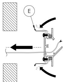
**Step 8; Fixture Assembly:** Connect the wires of Luminaire (C) to Low voltage cables of Driver (A). Then, gently insert the Luminaire (C) into Housing (B) until it snaps in properly. The wire
