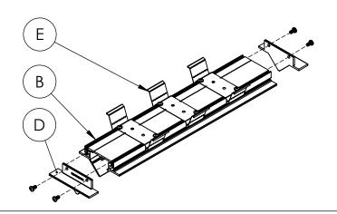
Step 4; Prepare the ceiling and housing for **installation:** Cut proper size opening into the ceiling. Cut out dimensions are listed below. Drill a 1/4" hole on the surface of housing along centerline of housing 2-1/2" away from one end as shown below.
