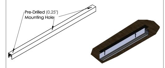
**Step 3:** (If single housing skip this step) Assemble Bent joiners. Place one bent joiner assembly and one straight joiner on each side of housing as seen below. Tigthen set screws using Allen Key.
