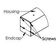
**Step 2:** Mount housing to surface using mounting screws (0.25" diameter pre-drilled holes). Mounting screw must be able to hold weight of the fixture)
