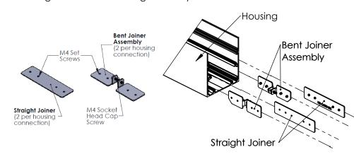
**Step 4:**(If single housing skp this step) Place next housing in ceiling end to end with first housing, slide joiners across housing seam so they are joining both housings. Tighten set screws on bent joiners, tighten the M4 Cap screw on bent joiners, tighten set screws on straight joiners. Mount housing. Repeat steps 3-4 until all housing are installed and mounted. Install endcap on last housing as seen in step 1.
