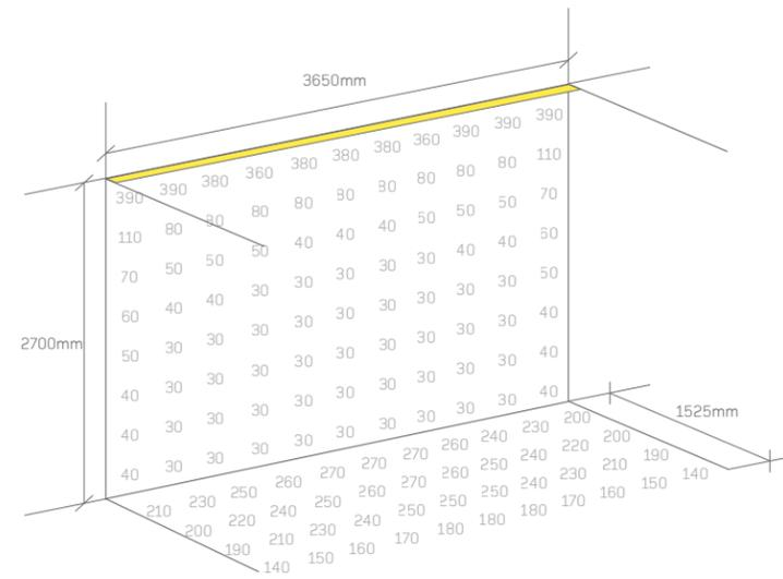
These diagrams indicate light levels to be expected on the wall and floor when using these luminaire types at various distances from the wall.
