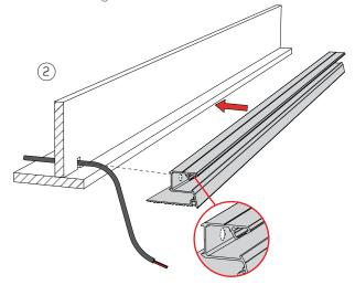
3. Feed the supplied cable grommet on to the cable to protect the cable from the drill hole.
