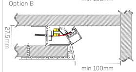
1. Construct a false ceiling (if applicable). Drill 10mm hole to feed 2 core 1.5-2.5mm<sup>2</sup> incoming DC power cable (not free issued). Expose 300-500mm of cable from wall
