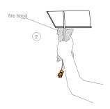
Drop the supply cable through luminaire hole cut-out
