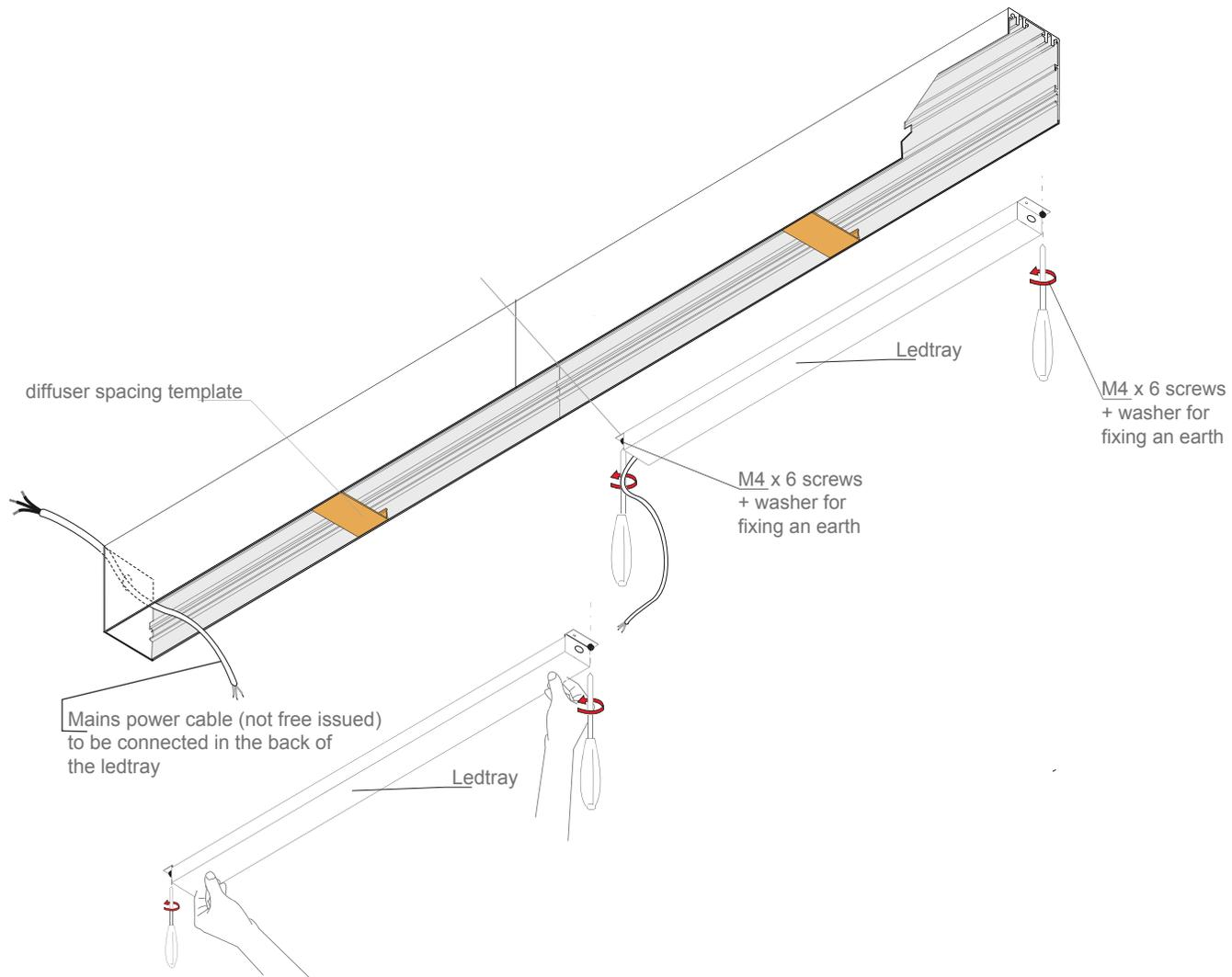
Do not remove the diffuser spacing template until the luminaire has been installed within the ceiling. If during installation the template falls from luminaire recheck diffuser aperture dimension 60mm, and return aperture to the required dimension. On completion of installation if diffuser spacing templates does not fit correctly/fall from luminaire then the diffuser will also not fit correctly, resulting in the failure of the luminaire.
