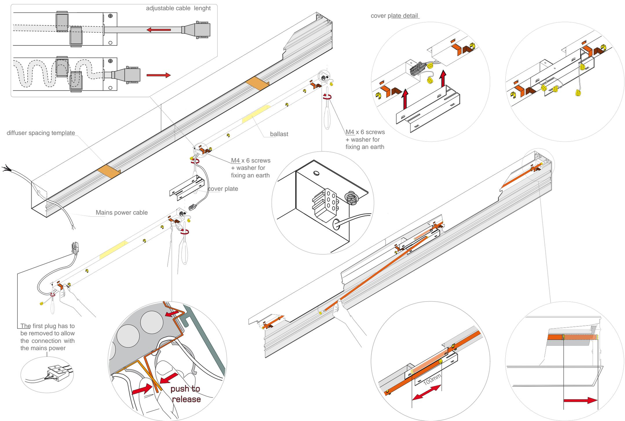
Do not remove the diffuser spacing template until the luminaire has been installed within the ceiling. If during installation the template falls from luminaire recheck diffuser aperture dimension 60mm, and return aperture to the required dimension. On completion of installation if diffuser spacing templates does not fit correctly/fall from luminaire then the diffuser will also not fit correctly, resulting in the failure of the luminaire.
