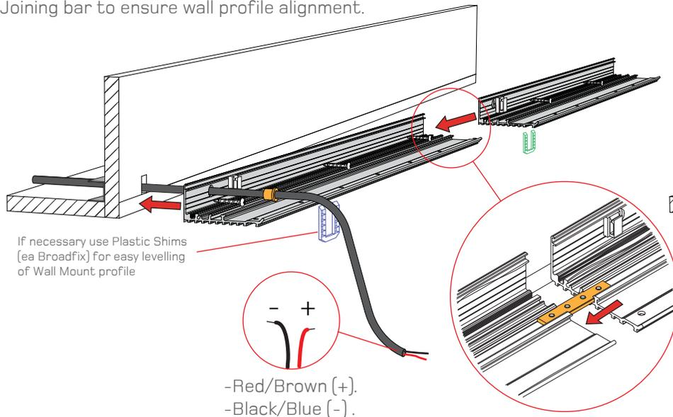
3. Follow step 2 from single module installation. Align multiple fixtures together. Loosen grub screws on the joint connector. Slide connector(s) across until it is equally spaced between the two fixtures. Ensure the 2 fixtures are securely joined together before fixing to wall profile.
