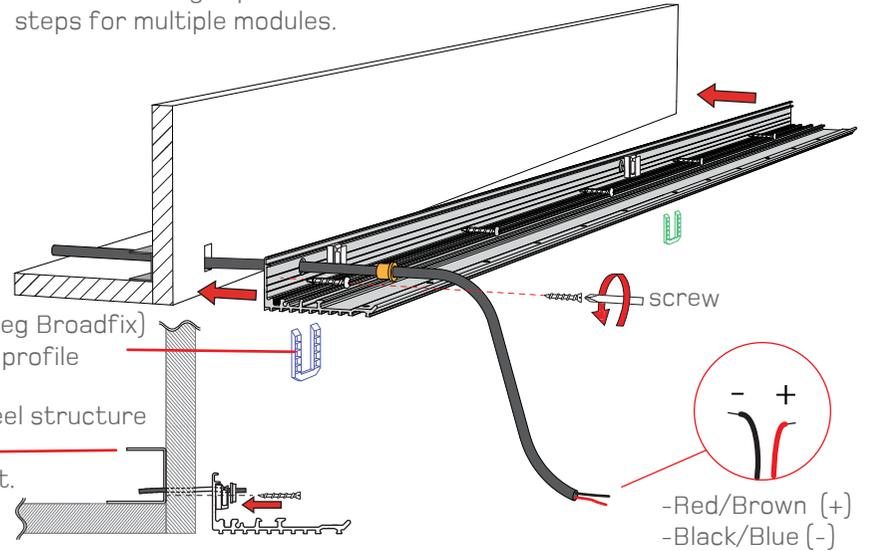
If necessary use Plastic Shims (eg Broadfix) for easy levelling of Wall Mount profile
