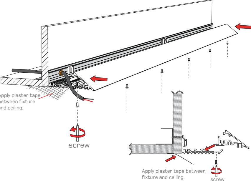
2. Align wall mount profile to wall and 10mm cut out hole. Mark on profile where the hole in the wall meets the profile and drill a hole in the profile so that they align. Ensure profile is straight and flush before securing in place. See alternative steps for multiple modules.
