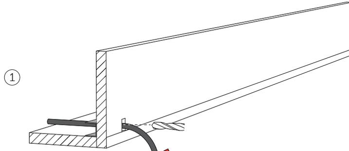
Drill 10mm hole to feed 2 core 1.5-2.5mm<sup>2</sup> incoming driver power cable (not free issued). Expose 30-50mm of cable from wall.
