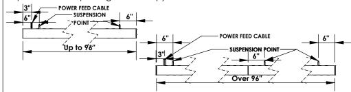
**Step 4:** Insert aircraft cable into power feed housing to suspend it at both locations. Adjust suspension to level the housing.
