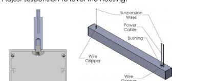
Step 6: (If single housing skp this step) Insert airfcraft cable into cable gripper on next housing. Then, slide joiners across housing seam so they are joining both housings. Tighten set screws on joiners. Repeat steps 5-6 until all housing installed and leveled. Install endcap on last housing as seen in step 1.
