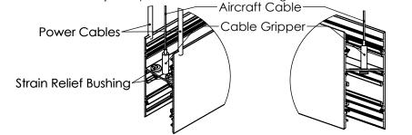
Step 6: (If single housing skp this step) Insert airfcraft cable into cable gripper on next housing. Then, slide joiners across housing seam so they are joining both housings. Tighten set screws on joiners. Repeat steps 5-6 until all housing are installed and leveled
