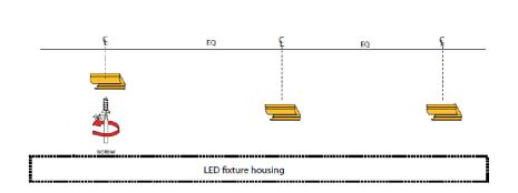
Magnetic Clip - Magnetic clips should already be pre-installled on fixture. Mount fixture directly to magnetic surface.
