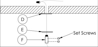
4C; Assembly of non-Powered Cable: Follow the same steps above for non-powered suspension cable at the other end of the Luminaire (B) except for electrical connection. Level the Luminaire and tighten the plastic set screws on Cable Holder (F).
