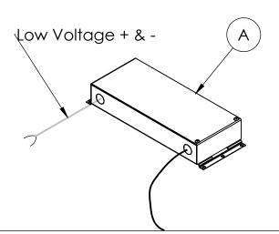
**Step 2**; **Prepare ceiling:** Mark the future position of the fixture on the ceiling. Then, drill holes in ceiling which correspond to suspension method of Luminaire (B). If it is plaster or tile ceiling, cut 1-1/4" holes with hole saw. If it is concrete or wood ceiling, holes should be adequately sized for the suspension cables. Pull low voltage cable of remote driver out through one of the holes.
