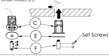
3C; Assembly of non-Powered Cable: Follow the same steps above for non-powered suspension cable at the other end of Luminaire (B) except for electrical connection. Level the Luminaire and tighten the plastic set screws on Cable Holder (F).
