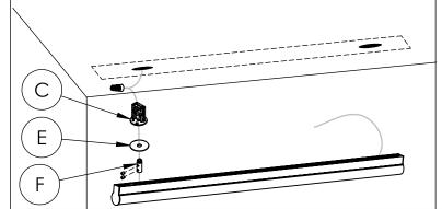
**3B**; Installation into Ceiling: Insert Plaster/Tile Canopy (C) with cable into ceiling hole, and tighten the captive screws under Canopy (C). This will lower and lock the claws onto the ceiling. Slide Cover Plate (E) and Strain Relief (F) up and screw it into Canopy (C). Adjust the cable length to the desired fixture height and secure by tightening the plastic set screw in the Strain Relief (F).
