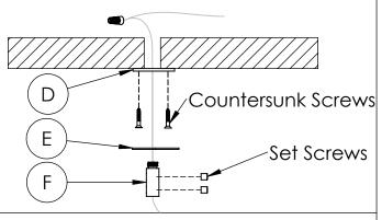
**4C**; Assembly of non-Powered Cable: Follow the same steps above for non-powered suspension cable at the other end of the Luminaire (B) except for electrical connection. Level the Luminaire and tighten the plastic set screws on Cable Holder (F).
