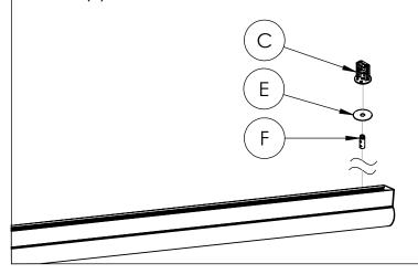
3D; Additional Suspension and Power Test: For fixtures longer than 60", install the center suspension the same way described in step 3C. Finally, power and test the Luminaire (B) for proper operation.
