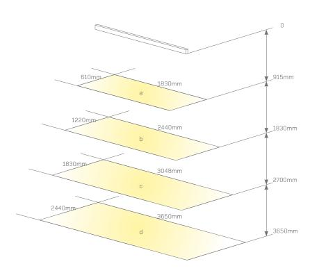
The diagram shows the average light level achieved across an area of the size shown, at the given distance from the luminaire.
